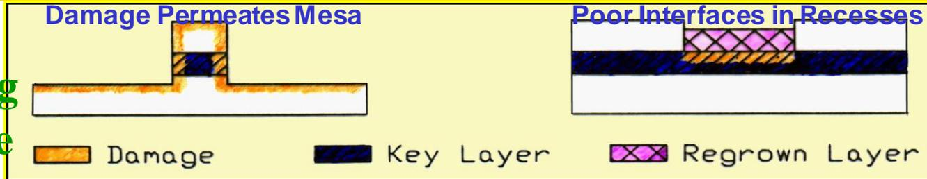
**Solution: low energy enhanced etching (LEEE=LE4) from DC discharge.**
